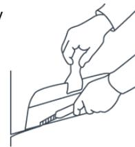
Processing on outside corners: Gently sand the fabric with wet sand paper, (> P 240), then wrap it around the corner and cut or use a corner bead.
