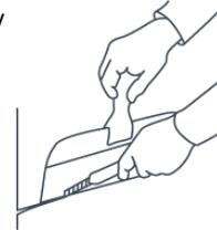
Processing on outside corners: Gently sand the fabric with wet sand paper, (> P 240), then wrap it around the corner and cut or use a corner bead.
